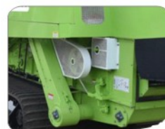
Provided cover for all moveable parts
