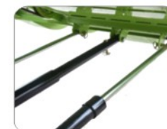
Cutter bar safety cylinder.
