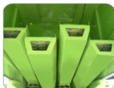
The four straw walker work in perfect coordination with the threshing mechanism which ensures optimum grain efficiency.
