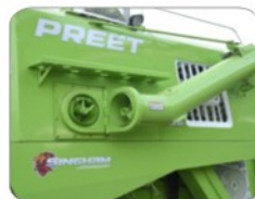
Grain tank can be emptied quickly with discharge tube. Discharge tube can be easily engage & Disengage with rods & latch assy.
