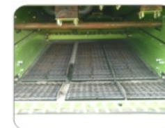
Well designed sieve section has a large cleaning area for optimum grain efficiency.
