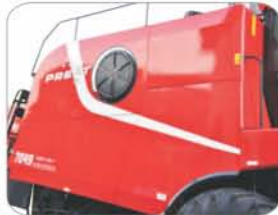
Bigger shields covering rotated parts with extra safety.
