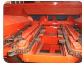
Large gathering chains and scoops that allows for large crop volumes to be conveyed to the auger.
