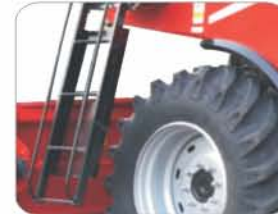
Ladder cover with sheet for safety purpose.
