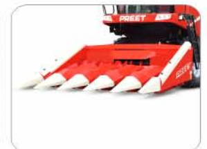
Broad cutter bar covering more cutting area. hardened & sharp edge cutting blade used. cutting blade drive thru. gear mechanism
