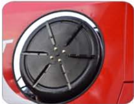
Engine cooling by clean air through rotating sieve equipped with additional fan.
