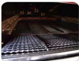
Large sieve area for optimum grain cleaning
