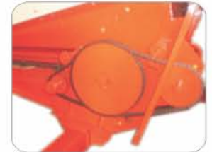
Auger drive with slip clutch for safety purpose.
